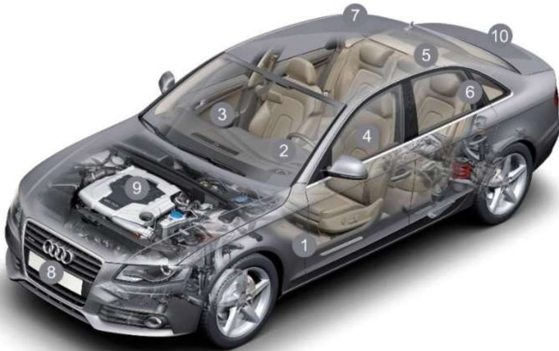
Figure 3: Car parts made of natural fibre composites
