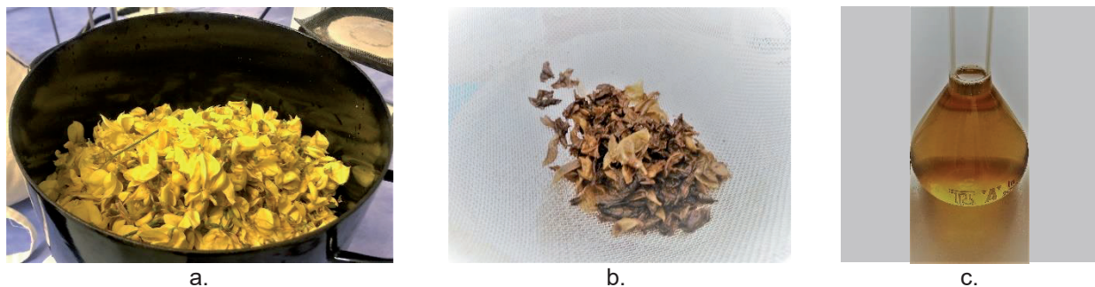
Figure 1: Extraction process in water: a. Spanish broom flowers; b. flowers after filtration; and c. an aqueous extract of Spanish broom flowers.
